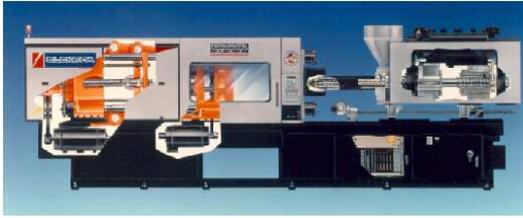
If the resin has an excessively high moisture content, this can result in surface defects, i.e. silver streaks, and impaired properties of molded parts. To ensure optimum part performance and prevent surface defects, LUPOY resins must be dried prior to processing, and moisture level maintained less than 0.05%. A dehumidifying hopper dryer is highly recommended.
